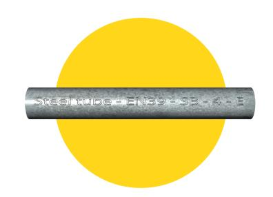
Scaffold tube should be made to EN39 and be galvanised steel. They should have a diameter of 48.3mm and a 3.2mm - 4.0mm wall thickness. Tubes should appear straight visually and not deviate by more than 15mm in any 3m length.
